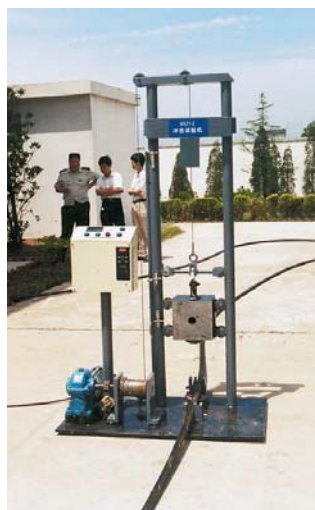
Shock test of SOFC
