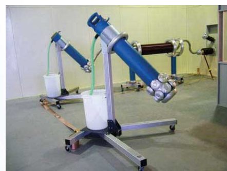
Partial discharge testing system
