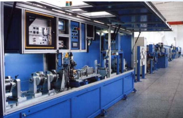
Layer Welding Line for Stainless Steel Tube Fiber Unit
