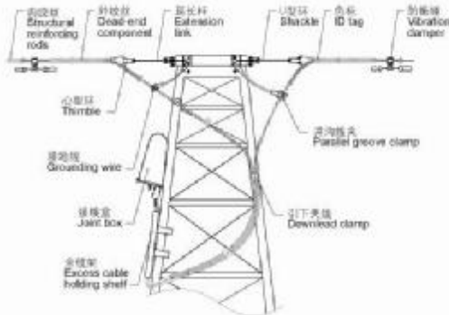
OPGW中间接续塔耐张线夹安装图 Installation Figure Of OPGW Dead-end On Joint Tower
