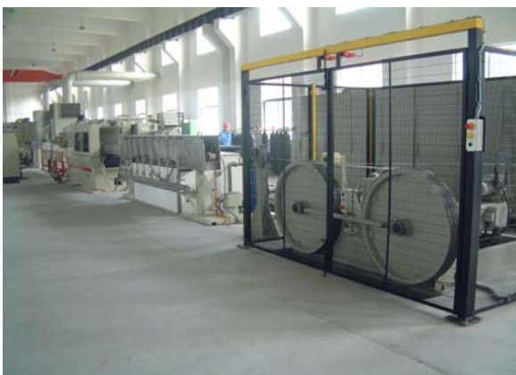
“Holton Conform 2000” continuous-extrusion and cladding machines imported from Britain
